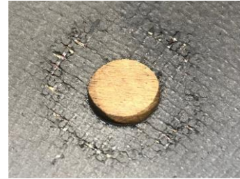
Type c) Breakage at bore area; the example pictures were obtained at the IFA and show different types of damage
