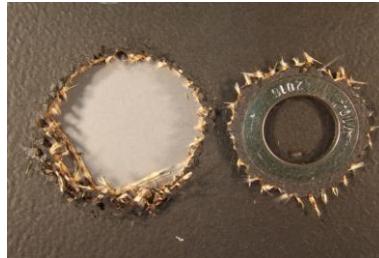
Type c) Breakage at bore area; the example pictures were obtained at the IFA and show different types of damage
