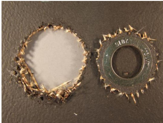
Type b) Breakage at bore area
